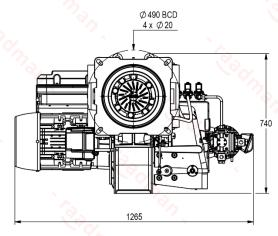
Suggested boiler flange diameter = 340 mm
